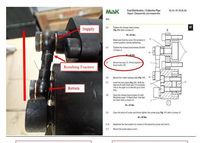
Photograph of misaligned fuel oil collective pipe, tightened to the point of fracture.
